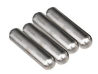
engineered for proper buoyancy for each particular application. In order to ensure product's measurement accuracy and working reliability, the size and weight of magnetic float need to be matched with measured fluid. Flap-11 Magnetic Level Indicator series products have a variety of magnetic floats. Flap-11 is suitable for medium density as low as 0.45g/cm<sup>3</sup>, which covers most mediums and conditions.
